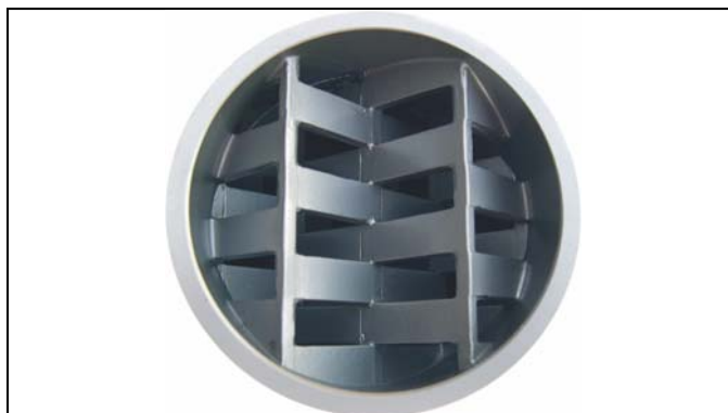
Figure #11: The SMB-R mixing elements are extremely strong due to their monolithic cast construction where the mixing bars are joined to each other and to the ring wall via a single molten metal pour.
